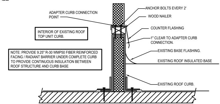
AHU-1 MECHANICAL ADAPTER CURB CONNECTION
