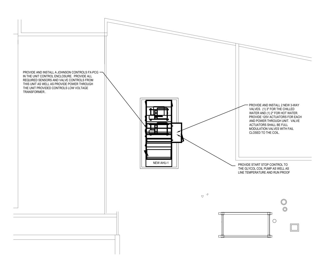
MECHANICAL ROOF CONTROLS GENERAL LAYOUT
