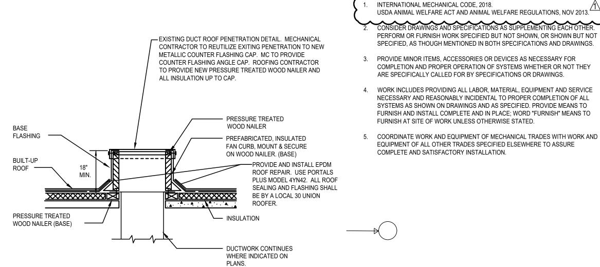
MECHANICAL DUCT PENETRATION DETAIL
