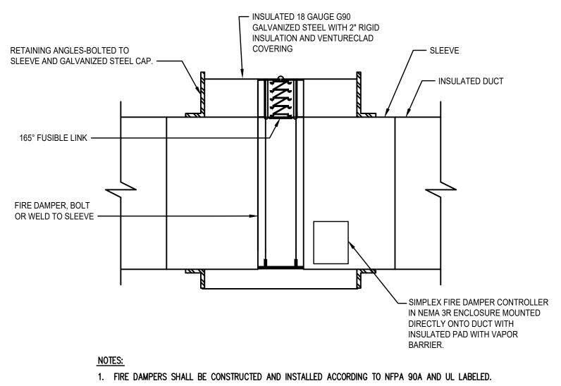
2. PROVIDE AN ACCESS PANEL FOR EACH FIRE DAMPER SECTION.
