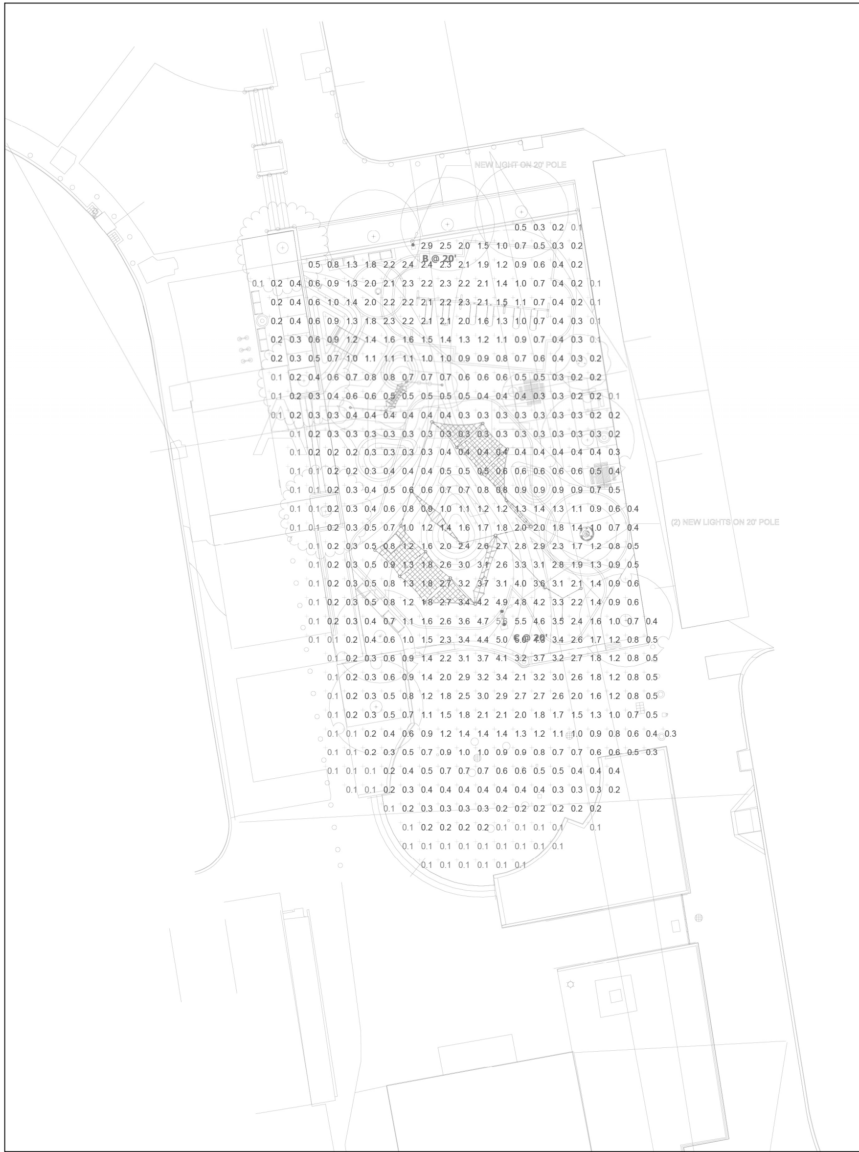
1 SITE 'E' LIGHTING FOOT CANDLES PLAN E201 SCALE: NOT TO SCALE
