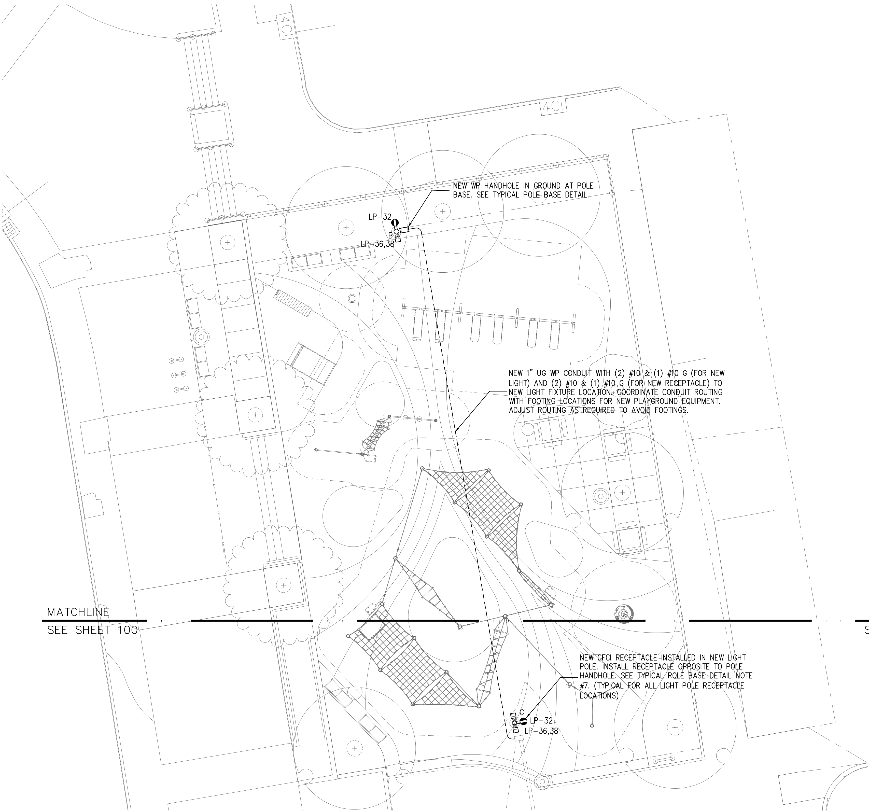
1 PARTIAL SITE 'E' NEW LIGHTING PLAN E101 SCALE: 1" = 10'-0"
