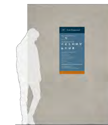
PLY.1.w Wall Mounted 1/2" thk panel
