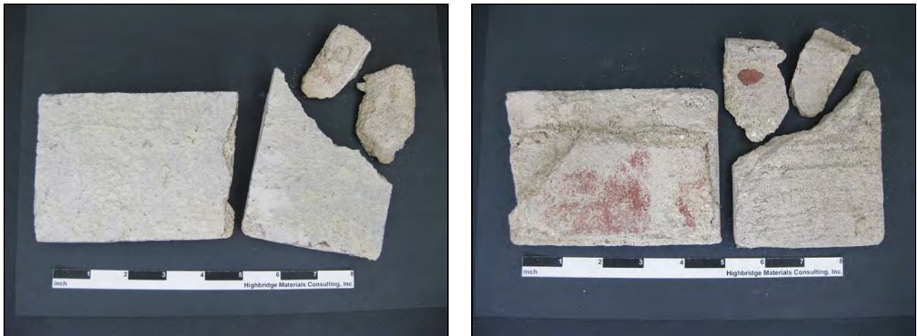
Figure 1: Photographs of the stucco sample provided to Highbridge for analysis. The left image shows the outer surface of the stucco, which is mostly covered with a dark brownish-gray skim coat and multiple coatings layers. There are small areas along the edge where some of the skim coat is fractured and the original pale yellow finish coat is visible beneath. The right image shows the inner surface of the stucco sample. This mostly shows the light brown scratch coat at the base of the stucco.
