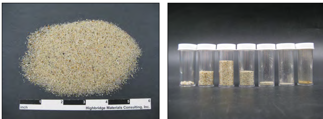
Figure 3: Photographs illustrating the sand sample extracted from the finish coat. The total extraction is shown at left. The sand is uniform with a light yellowish-brown color and fine, dark glauconite flecks. At right, the sand is shown after gradation through a standard sieve stack. The sand is broadly-graded and somewhat fine-grained.
