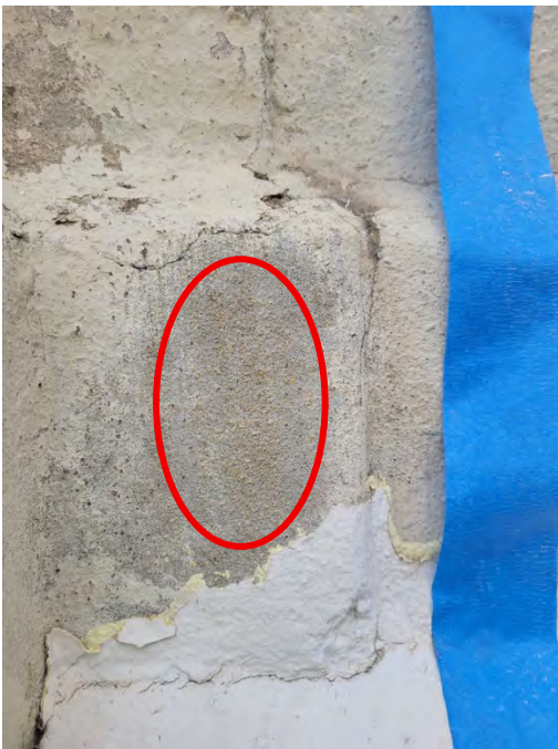
Figure 16. Test location of the calcium carbonate micro-abrasive media, after testing. Calcium carbonate micro-abrasive media was tested on a small area (circle). It successfully removed the remaining overpaint to reveal the brownish gray stucco skim coat.
