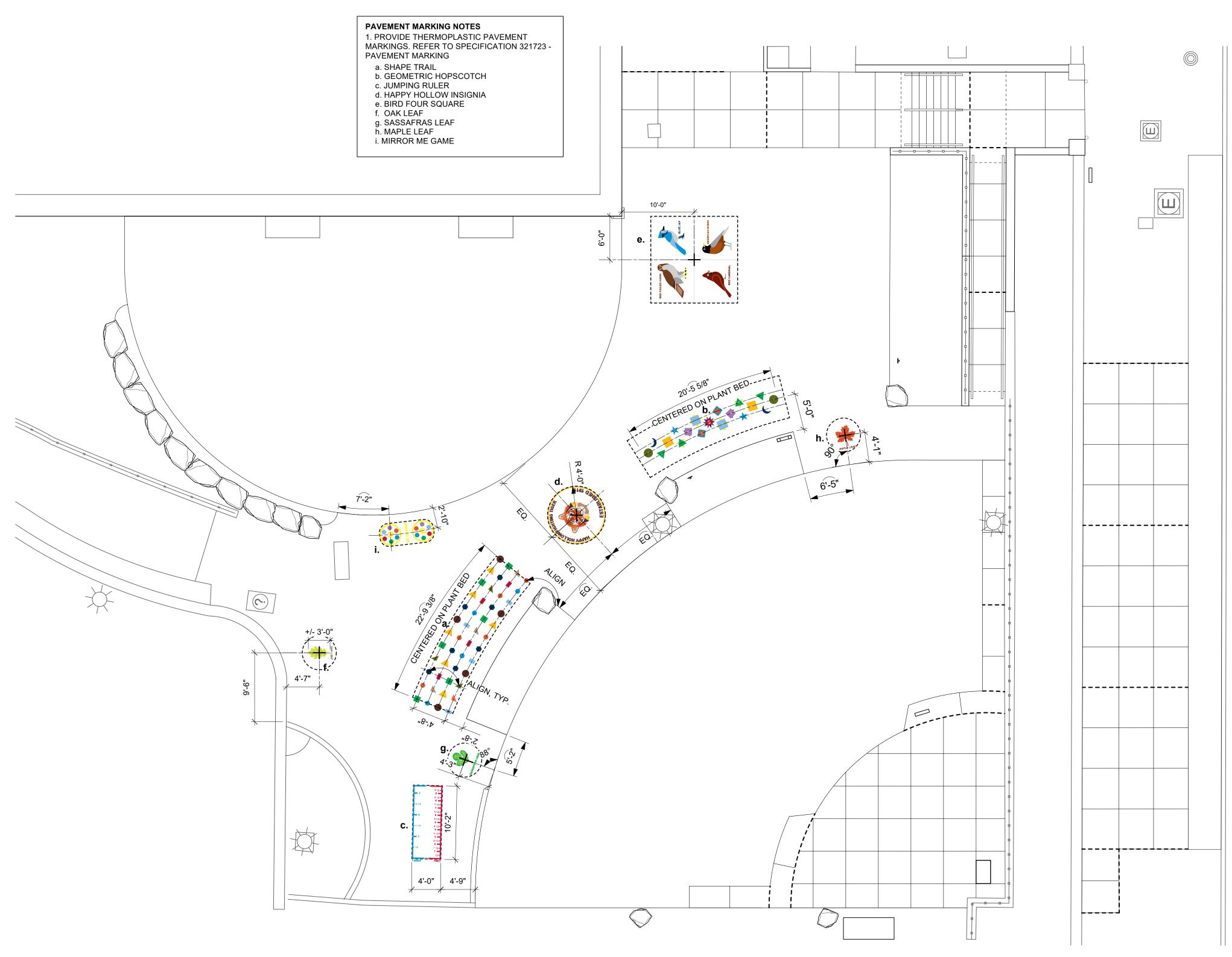
2 DETAIL ENLARGEMENT PLAN - PAVEMENT MARKINGS L6.4 Scale: 1/8" = 1'-0"
