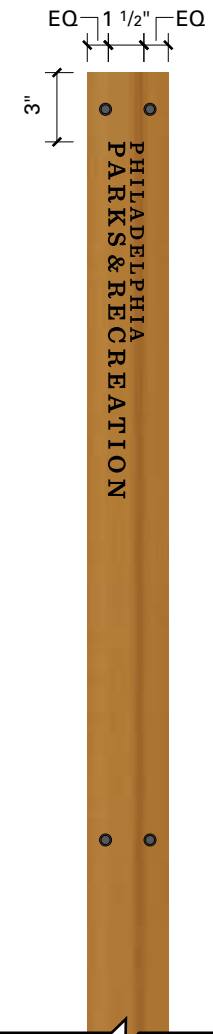
Graphic Layout - Wood side panel Scale: 1 1/2"=1'
