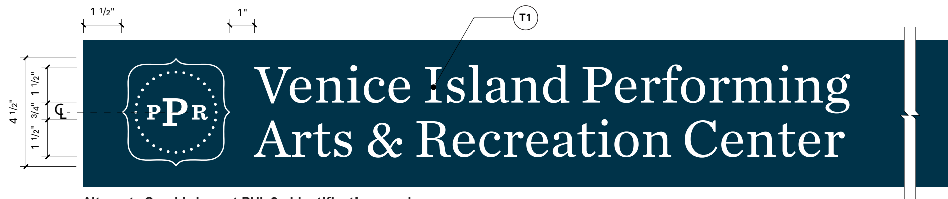
Alternate Graphic Layout BUL.2 - Identification panel Scale: 3"=1'
