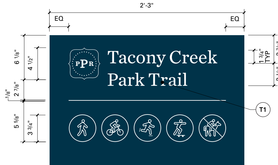
Graphic Layout - TID.1.p Upper Panel Scale: 1 1/2"=1'
