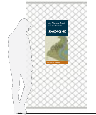
TID.1.f Fence Mounted 1/2" thk panel
