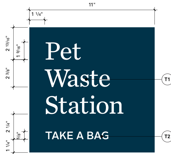
Graphic Layout - SID.3.p Upper Panel Scale: 3"=1'
