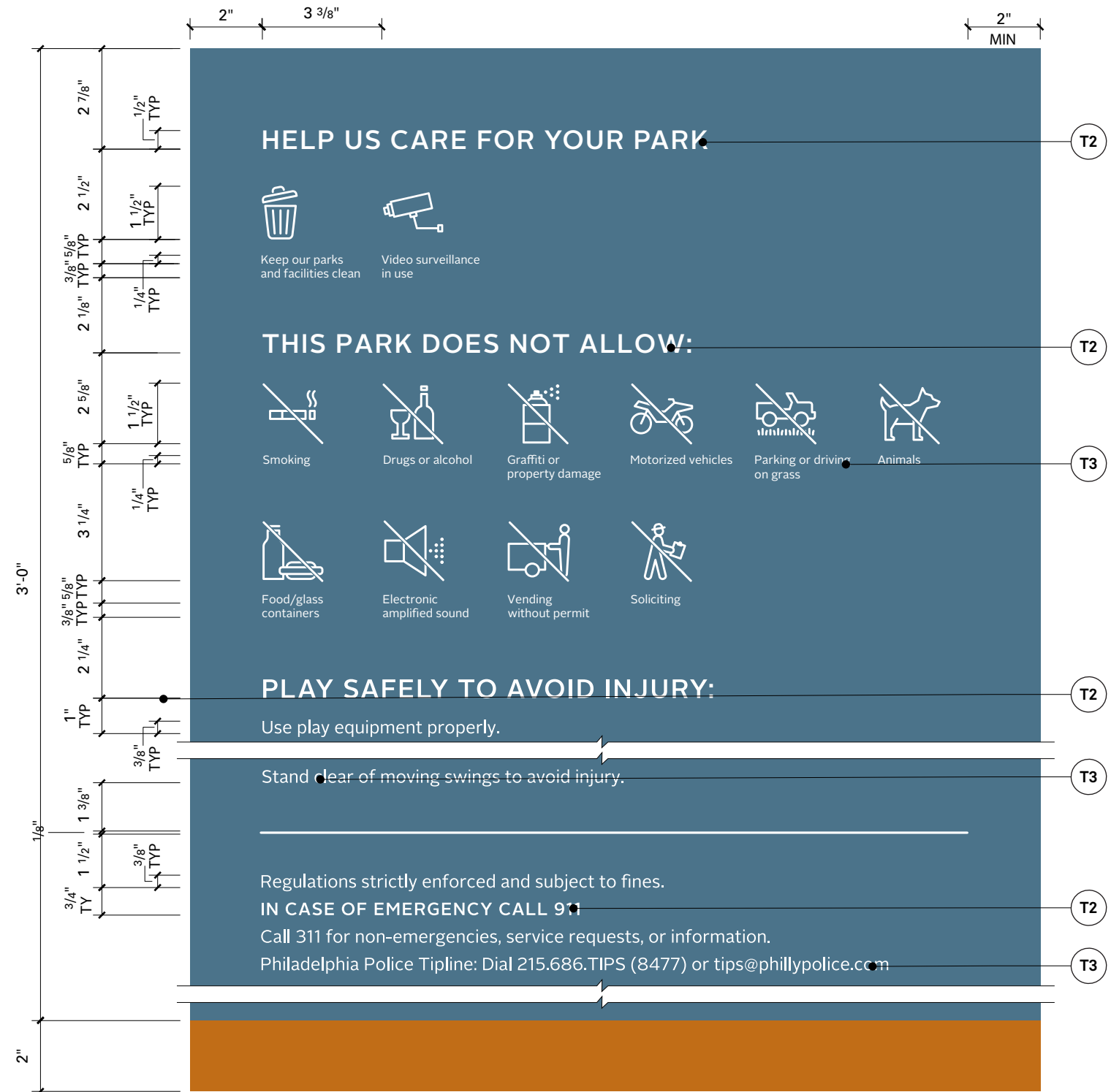
Graphic Layout - PLY.1 Regulatory panel Scale: 3"=1'
