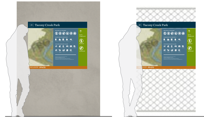
PID.3.w Wall Mounted 1/2" thk panel
