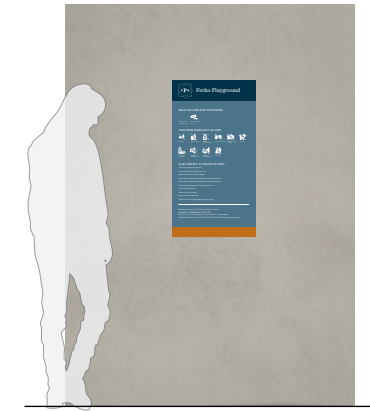
PLY.1.w Wall Mounted 1/2" thk panel
