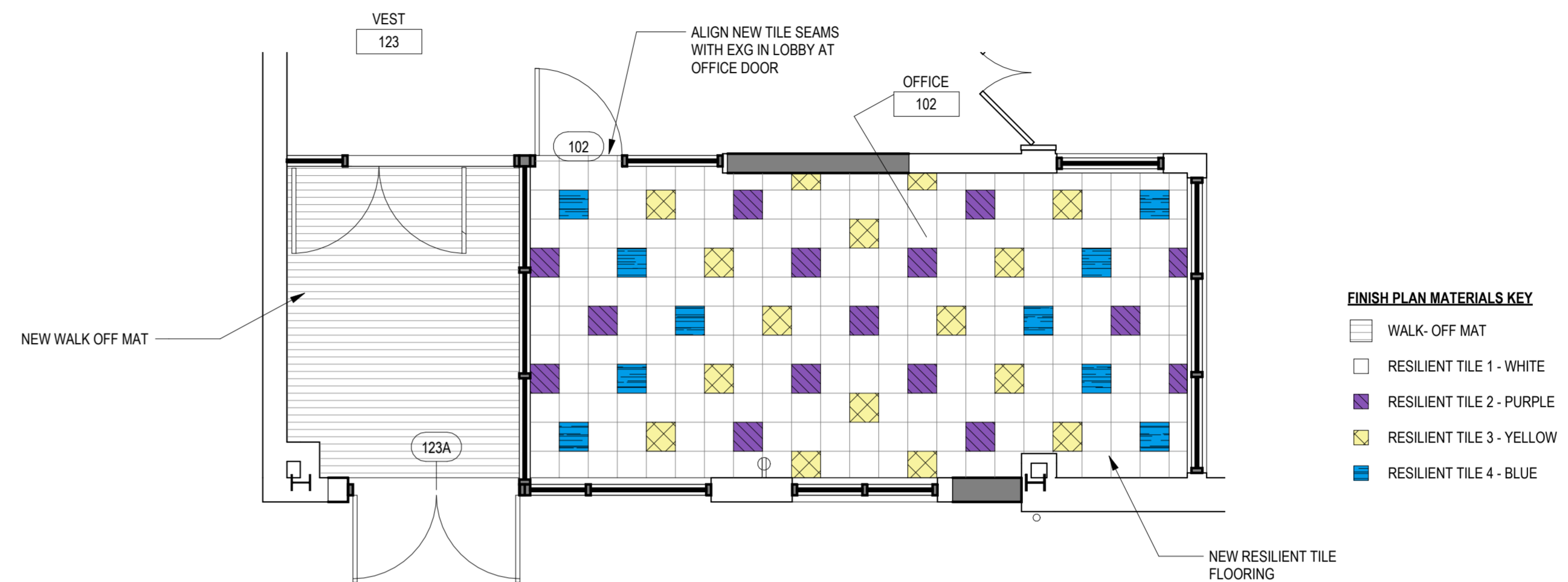
3 ENLARGED FINISH PLAN A9.0(1) 1/4" 1'-0"
