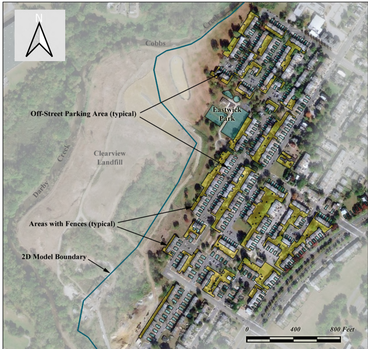
Figure 14: Manning's N Adjustments in Terrestrial Overflow Area
